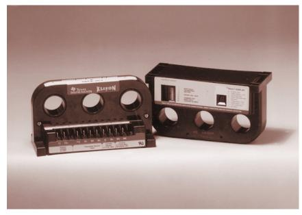
individual applications with a "Must Hold" current range from 25 - 225 Amps. The trip curves allow for starting inrush currents normally seen in Y-delta , part winding, and double delta wound motors without nuisance tripping.
